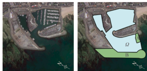
Fig. 3. Illustration of La Turballe Port. Left: The port in its initial state. Right: The port with the two additional structures considered in this study: Mole A and Jetty B.
