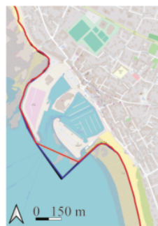
Fig. 12. Results of the long term morphodynamic simulation with and without the proposed structures. The simulations without the redesign of the port are given by the dotted lines: yellow is the initial shoreline and red is the shoreline after the 30-year simulation. The simulations incorporating the redesign of the port are given by the solid lines: black is the initial shoreline and blue is the shoreline after the 30-year simulation.
